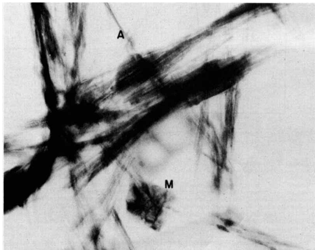
Figure 10 —Electron photomicrograph of sodium-treated attapulgite showing the elongate lath-shaped particles (A) that are characteristic of attapulgite and the irregularly shaped aggregates (M) believed to be the montmorillonite-like impurity (magnification = 30,000 \times ).
